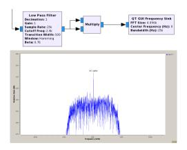
Power 2 of the signal has DC spike  $\Rightarrow$  BPSK For QPSK, we would need to go to 4th power
